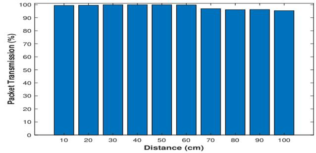
Fig. 13: Packet success rate during transmission with distance
