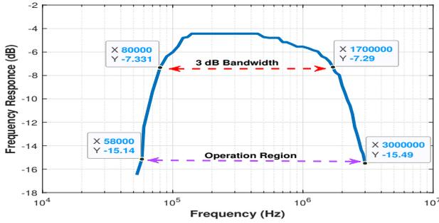
Fig. 10: Frequency response of modified receiver design
