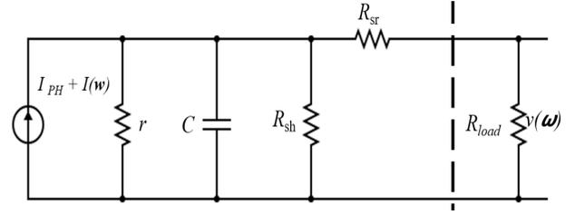
Fig. 3: AC model of solar panel
