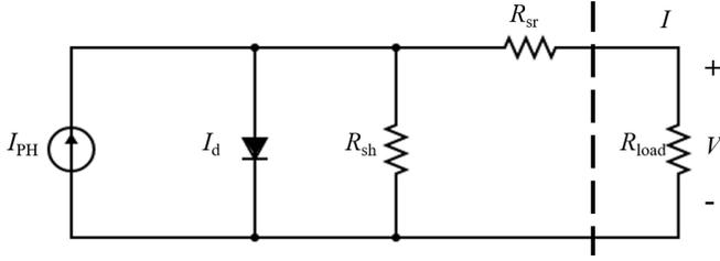
Fig. 2: Electrical equivalent model of solar panel
