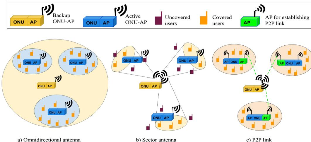
Fig. 2. Clustered architecture of active ONU-APs, where backup ONU-AP is equipped with a) Omnidirectional antenna, b) Sector antenna, and c) Parabolic grid antenna for P2P link.
