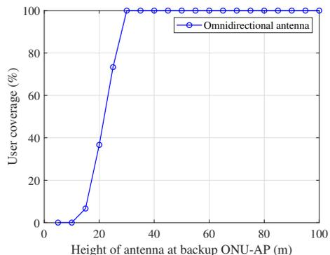
Fig. 7. User coverage (%) with respect to height of antenna at backup ONU-AP equipped with omnidirectional antenna
