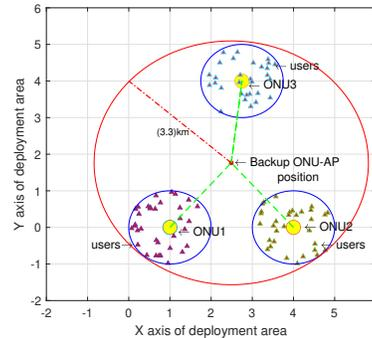
Fig. 3. Optimal position for backup ONU-AP in case of uniform distribution of users
