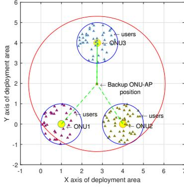
Fig. 4. Optimal position for backup ONU-AP in case of non-uniform distribution of users
