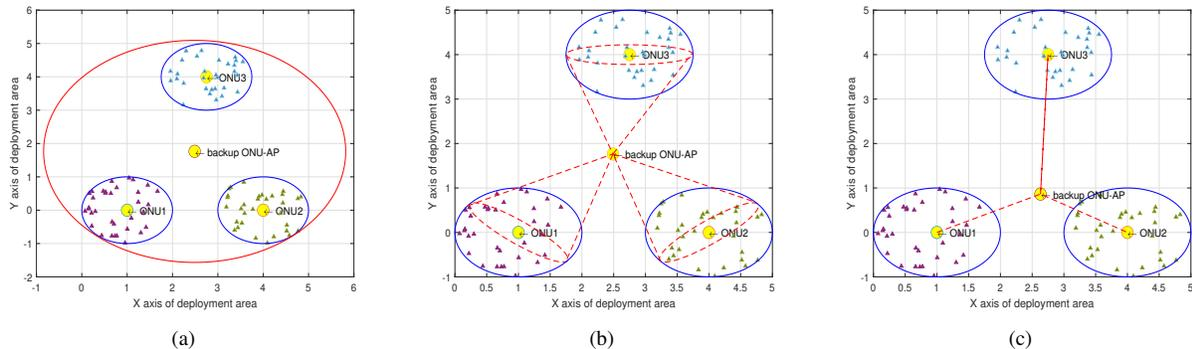
Fig. 6. Placement of backup ONU-AP for different antenna configurations a) Omnidirectional Antenna, b) Sector Antenna, and c) P2P link.
