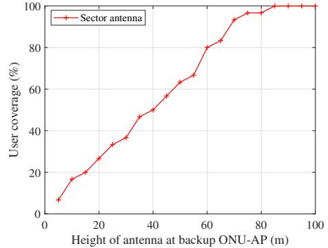
Fig. 9. User coverage (%) with respect to height of antenna at backup ONU-AP (in case of sector antenna)
