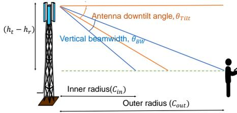
Fig. 8. Illustration inner and outer radius of ellipsoid region of backup ONU-AP, when it is equipped with sector antennas
