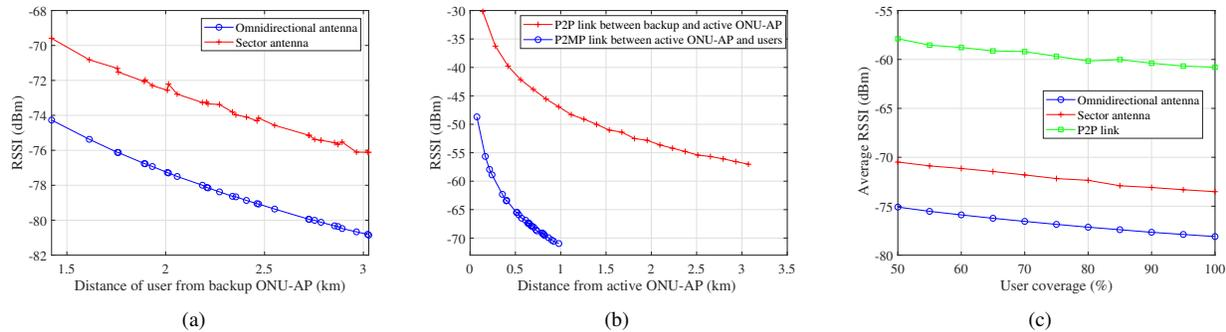
Fig. 11. RSSI of the users with respect to distance, when backup ONU-AP is connected to active ONU-AP via (a) omnidirectional antenna and sector antenna, (b) P2P link, and (c) Average RSSI (dBm) with respect to user coverage (%)
