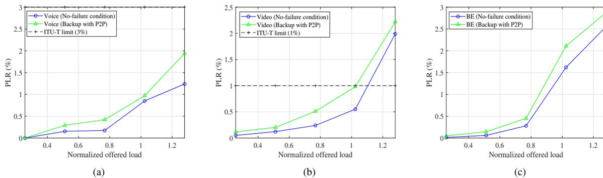
Fig. 14. PLR with respect to normalized offered load for a) Voice, b) Video, and c) BE traffic.
