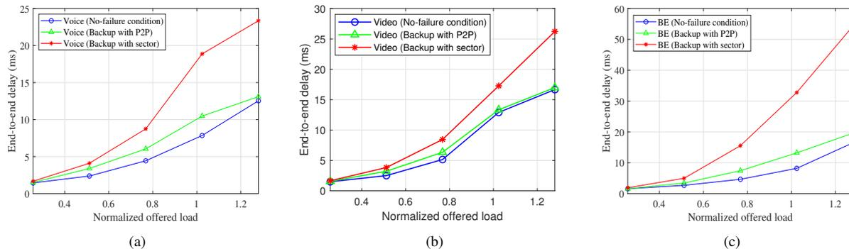
Fig. 13. End-to-end delay with respect to normalized offered load for a) Voice, b) Video, and c) BE traffic.
