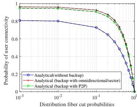
Fig. 16. Probability of users connectivity with respect to distribution fiber cut probabilities (where ONU and AP's failure probability is  $10^{-1}$ ) is considered
