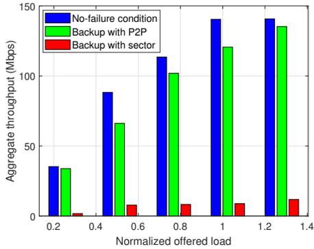
Fig. 12. Aggregate throughput with respect to normalized offered load
