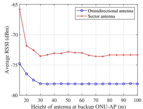
Fig. 10. Average RSSI (dBm) with respect to height of antenna at backup ONU-AP (m).
