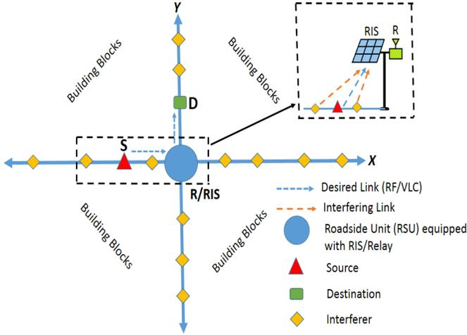
Fig. 2: Abstraction system model for vehicular communications involving a source  $S$ , relay  $R$ /RIS and a destination  $D$  in presence of one dimensional Poisson field of interference.
