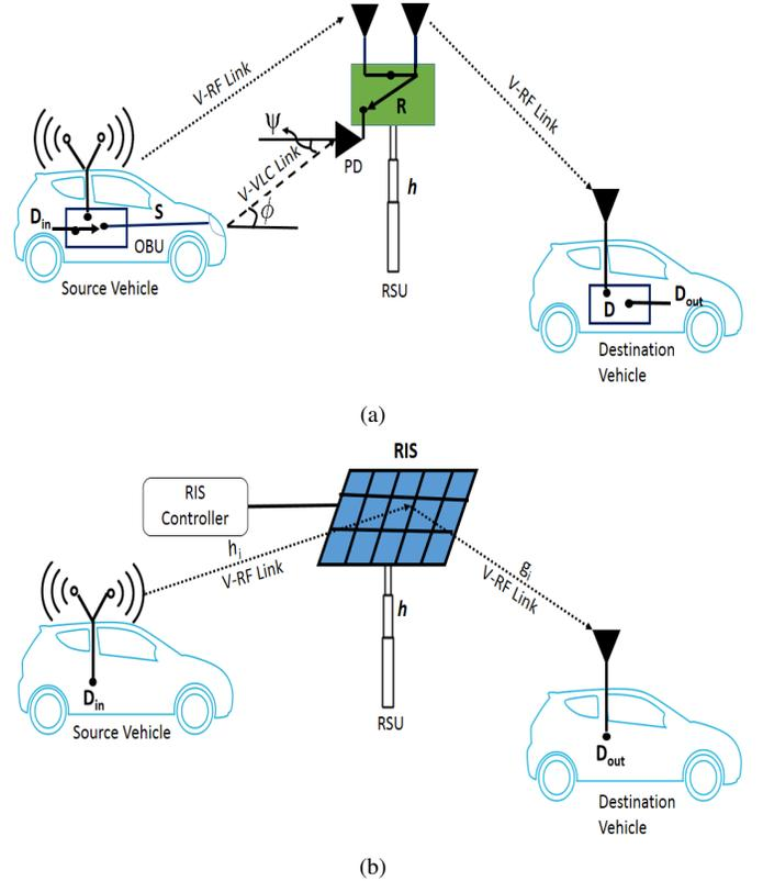
Fig. 3: Illustration of proposed V2X deployment strategies: (a) Hybrid V-VLC/V-RF scheme and (b) V-RF with RIS scheme.
