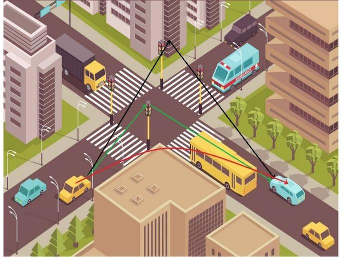
Fig. 1: Illustration of road intersection scenario where vehicles in blocked line-of-sight (solid red line) can communicate via Hybrid V-VLC/V-RF with relaying (solid green line) and V-RF with RIS (solid black line).
