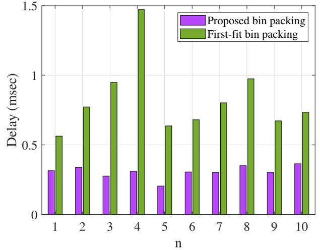
Fig. 5. Delay at  $\text{ONU}_n$  after switching minimization
