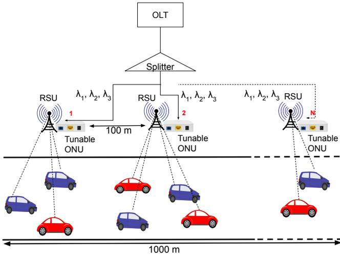
Fig. 1. System Architecture for the considered FiWi-V2I network
