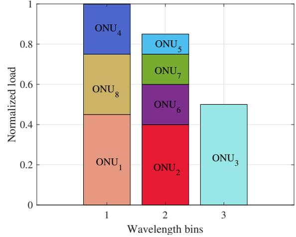
Fig. 4. Wavelength Allocation using proposed bin packing
