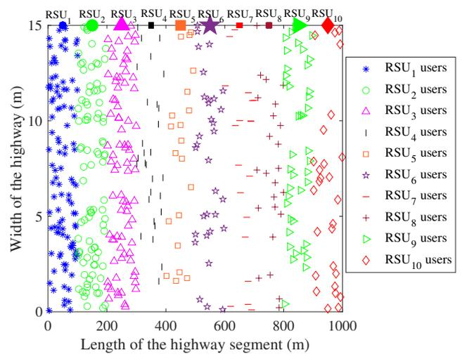
Fig. 2. Association of vehicles with RSUs based on throughput
