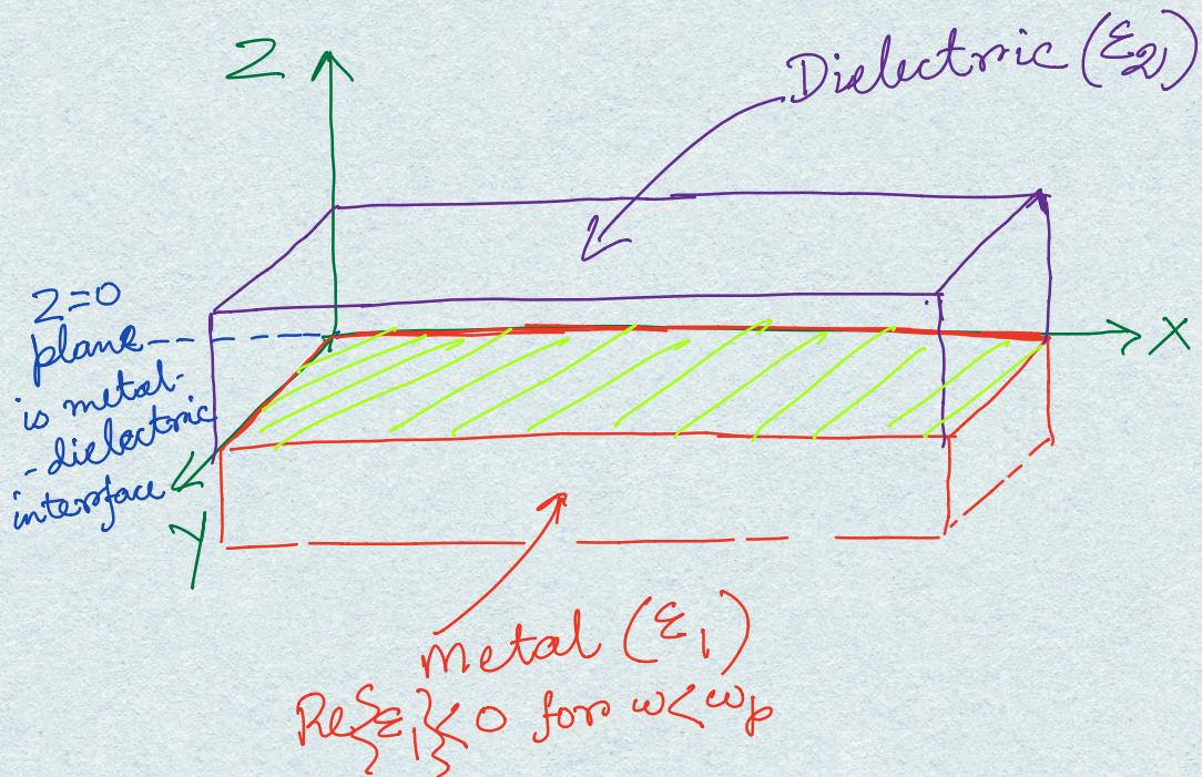
We are interested in a solution of the wave eqn (1), where the fields will decay exponentially (along  $Z$  direction) on either sides of the interface but the wave propagates along  $X$ -direction (i.e. evanescent along  $Z$  but propagating along  $X$ )
