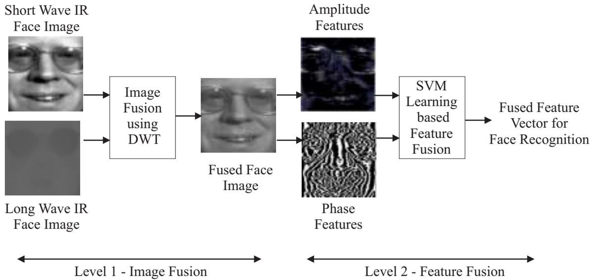
Fig. 6. Two-level hierarchical fusion of multi spectral face images
