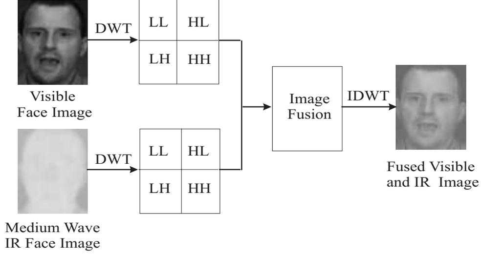
Fig. 4. Multispectral image level fusion of visible and medium-wave infrared face images
