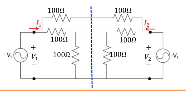
This situation still preserves the **symmetry** of the circuit— **somewhat.** The **voltages** and **currents** in the circuit will now posses **odd symmetry**—they will be **equal but opposite** (180 degrees out of phase) at symmetric points across the symmetry plane.
