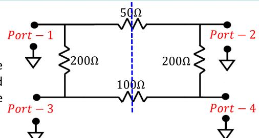
Continuing for all elements of the permutation, for this symmetric circuit, the s-matrix must have this form:
