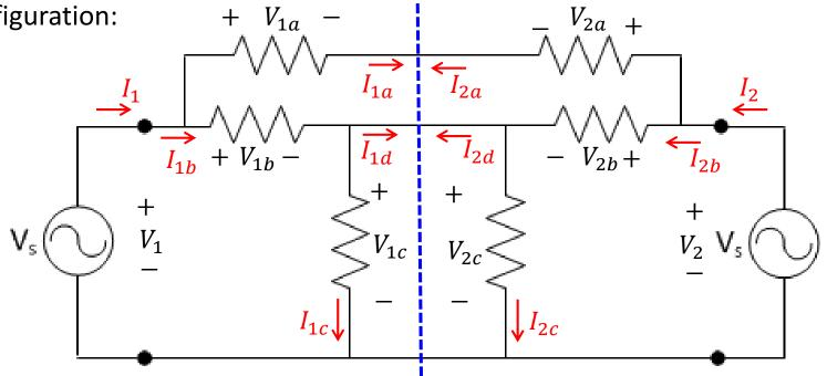
• Since this circuit possesses **bilateral** (reflection) symmetry  $(1\rightarrow 2, 2\rightarrow 1)$ , symmetric currents and voltages must be equal:
