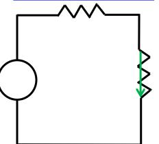
Just like section 2, the contour moves through a **resistor**. The contour integral for this section is thus equal to the potential difference across this **second** resistor, which we denote as  $V_2$ :
