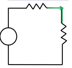
Just like section 1, the contour follows a **wire**, and thus the electric field long this section of the contour is **zero**, as is the potential difference between point c and point d.
