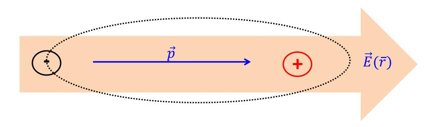
As a result, atoms/molecules form **electric dipoles** when an electric field is present!
