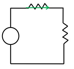
In this section, the contour moves through the first **resistor**. The contour integral along this section therefore allows us to determine the electric **potential difference** across this resistor. Let's denote this potential difference as  $V_1$ :
