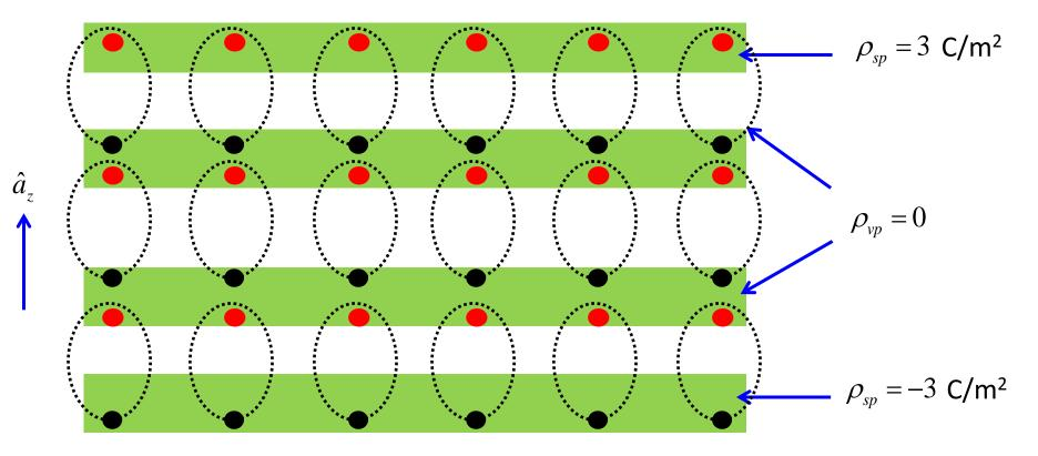
• In the **middle** of the dielectric, there are **positive** charge layers on top of **negative** charge layers. The two add together and **cancel** each other, so that equivalent **volume** charge density is **zero**.
