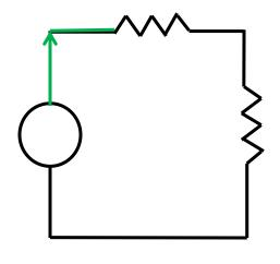
In this section, the contour follows the **wire** from the voltage source to the first resistor. We know that the electric field in a perfect conductor is **zero**, and likewise in a good conductor it is **very small**. Assuming the wire is in fact made of a **good conductor** (e.g. copper), we can approximate the electric field **within** the wire (and thus at **every** point along section 1) as **zero** (i.e.,  $\vec{E}(\vec{r}) = 0$ ). Therefore, this first integral equals zero!
