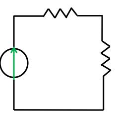
This **final** section of contour  $C_1$  extends through the **voltage source**, thus the contour integral of this section provides the electric potential difference between the two terminals of the this voltage source (i.e.,  $V_f - V_a$ ). By **definition**, the potential difference between points a and f is a value of V volts (i.e.,  $V_a - V_f = V$ ). Therefore, we find that the contour integral of section 6 is:
