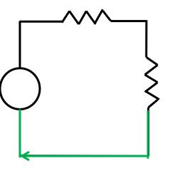
Again, the contour follows a conducting wire—and again, the electric field along the contour and the potential difference across it are both zero:
