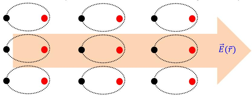
• We therefore define an average dipole moment, per unit volume, called the Polarization Vector  $\vec{P}(\bar{r})$ .
