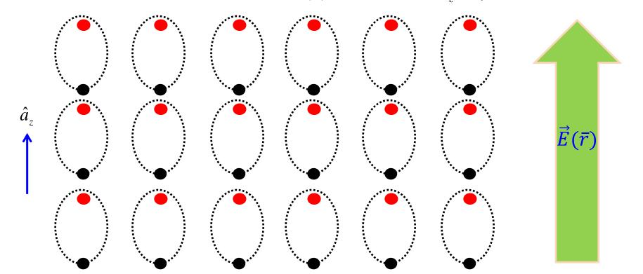
Note since the polarization vector is a constant, the equivalent volume charge density is zero:
