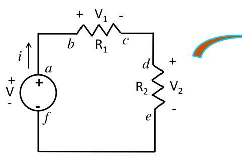
We find that if the **voltage source** is on (i.e.,  $V \neq 0$ ), there will be electric potential differences (i.e., voltage) between different points of the circuit. This can **only** be true if **electric fields** are present!
