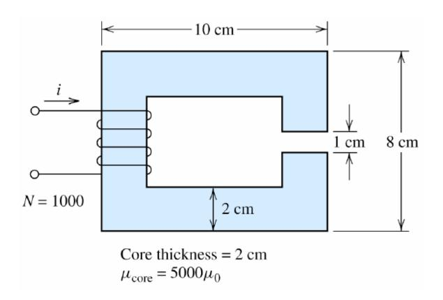
Determine the current required to establish a flux density of 0.5T in the air gap
