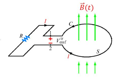
$$V_{emf}^{tr} = V_{12} = -\int_{S} \frac{\partial \overrightarrow{B}}{\partial t} . ds$$
