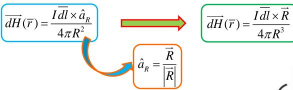
• This direction of  $\overrightarrow{dH}(\overline{r})$  can be obtained from right-hand rule: right-hand thumb points in the direction of current and the right hand fingers encircle the wire in the direction of  $\overrightarrow{dH}(\overline{r})$ .
