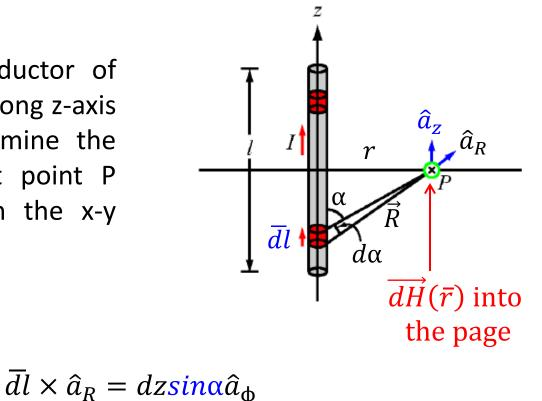
where lpha is the angle between  $\overline{d}l$  and  $\widehat{a}_R$
