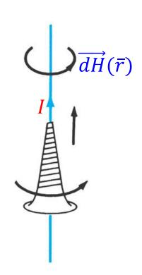
• It is a standard practice to represent the direction of magnetic field intensity  $\vec{H}(\bar{r})$  (or current I) by a small circle with a dot or cross depending on whether  $\vec{H}(\bar{r})$  (or I) is out of or into the page.
