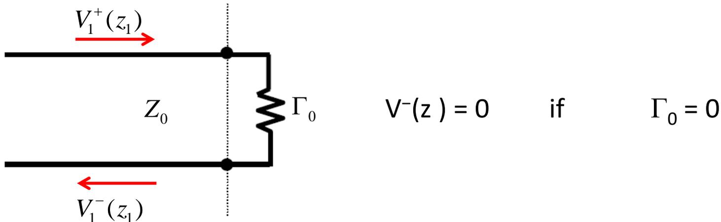
In this original case, the wave **incident** on the load is  $V^+(z)$  (**plus** direction), while the **reflected** wave is  $V^-(z)$  (**minus** direction).
