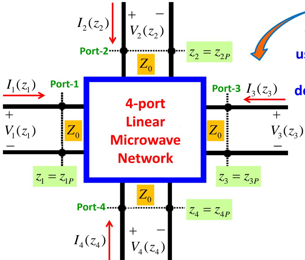
This can be characterized using admittance matrix – if currents are taken as dependent variables instead of voltages
