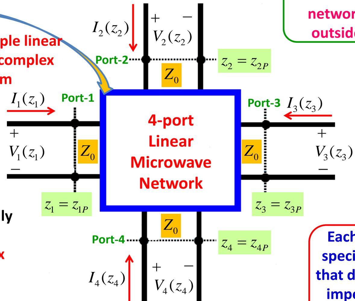
Either way, the network can be fully described by its impedance matrix
