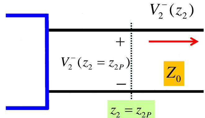
The complex ratio between  $V_1^+(z_1 = z_{1P})$  and  $V_2^-(z_2 = z_{2P})$  is known as the **scattering parameter  $S_{21}$**
