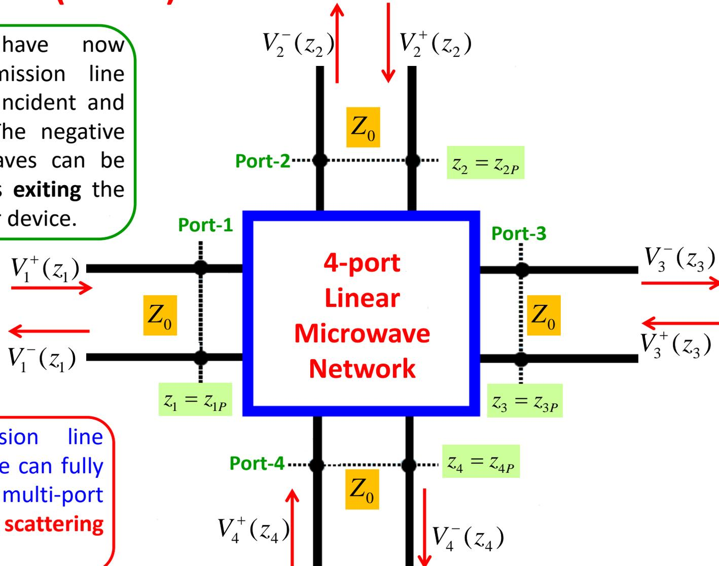
Viewing transmission line activity this way, we can fully characterize a multi-port device by its **scattering parameters!**
