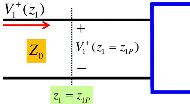
Say we measure/determine the voltage of the wave flowing **into port 1**, at the port 1 plane (i.e., determine  $V_1^+(z_1 = z_{1P})$ ).
