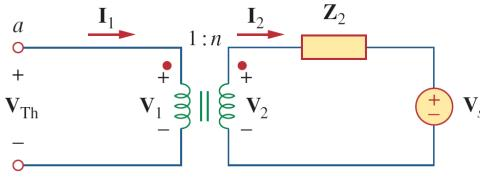
• First, obtain  $V_{TH}$  as open-circuit voltage at terminals a-b.
