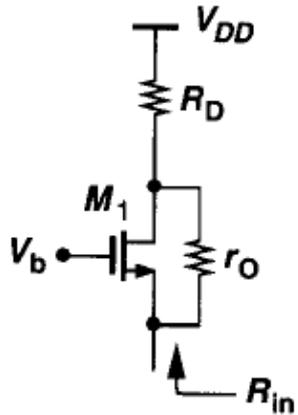
$$\therefore R_{in} = \frac{R_D + r_o}{1 + (g_m + g_{mb})r_o} \approx \frac{R_D}{(g_m + g_{mb})r_o} + \frac{1}{(g_m + g_{mb})}$$
