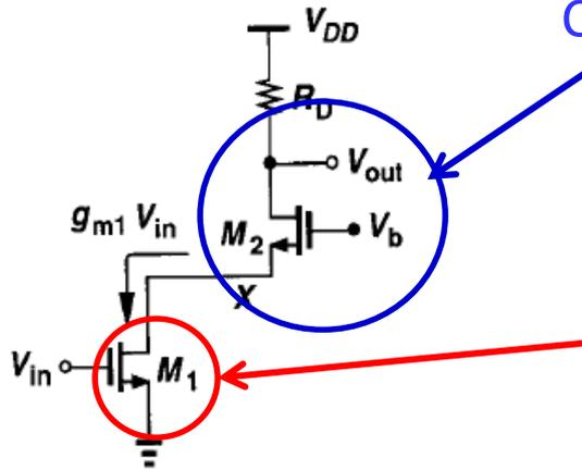
Cascode device (in CG) → in saturation → routes the current generated by main device to  $R_D$
