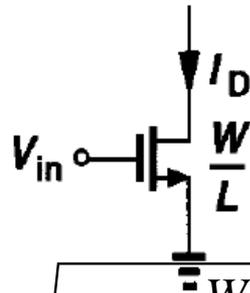
$$A_v \approx -g_m r_o = \sqrt{2\mu_n C_{ox} \frac{W}{L} I_D} \frac{1}{\lambda I_D}$$
