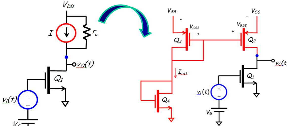
Transistors  $Q_2$ ,  $Q_3$ , and  $Q_4$  form the **current mirror** that acts as the **current source**. Note that transistor  $Q_4$  is an **enhancement load**—it acts as the **resistor** in the current mirror circuit.
