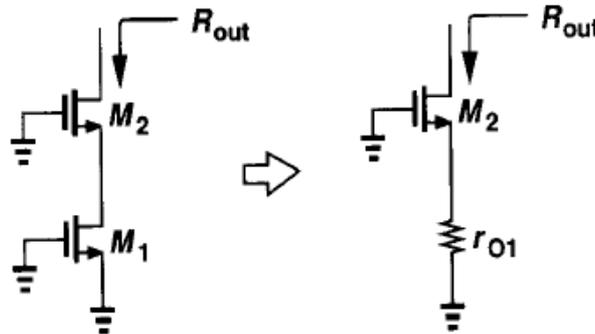
$$R_{out} \approx (g_{m2} + g_{mb2})r_{o2}r_{o1}$$
