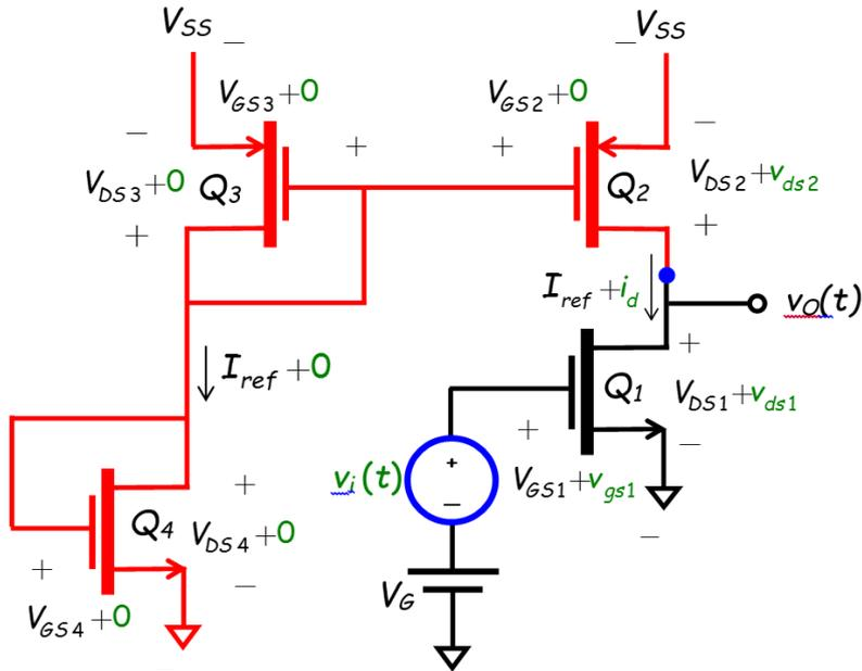
**Q:** But wait! **How** can there be a small-signal **drain current**  $i_{d2}(t)$  through transistor  $Q_2$ , **without** a corresponding small-signal  $v_{gs2}(t)$  **gate-to-source voltage**?
