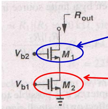
Cascode Transistor (CG Stage): always in saturation and is the main device that provides a constant current source
