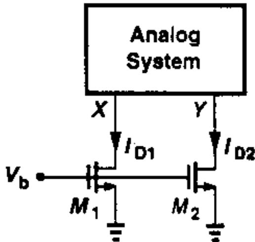
Q: determine the resulting difference between  $I_{D1}$  and  $I_{D2}$  if  $\lambda \neq 0$
