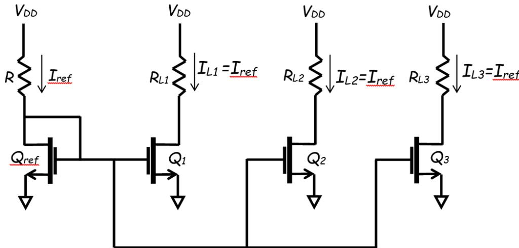
This circuit is particularly useful in integrated circuit design, where **one** resistor  $R$  is used to make **multiple** current sources.
