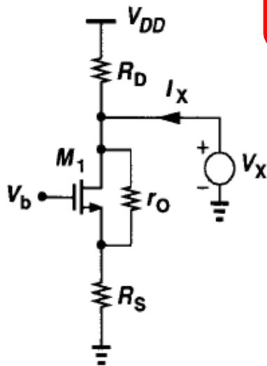
$$R_{out} = \frac{V_X}{I_X} = \left\{ [1 + (g_m + g_{mb})r_o] R_S + r_o \right\} \parallel R_D$$
