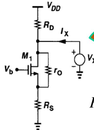
$$R_{out} = \left\{ \left[ 1 + (g_m + g_{mb})r_o \right] R_S + r_o \right\} \parallel R_D$$
