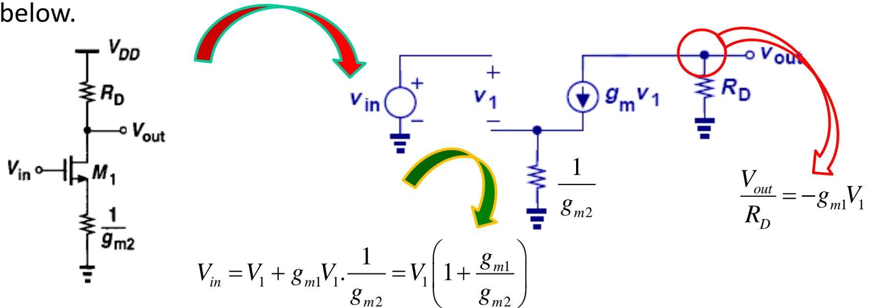
**Simplification gives:**  $V_{out} = -g_{m1} V_1 R_D$
