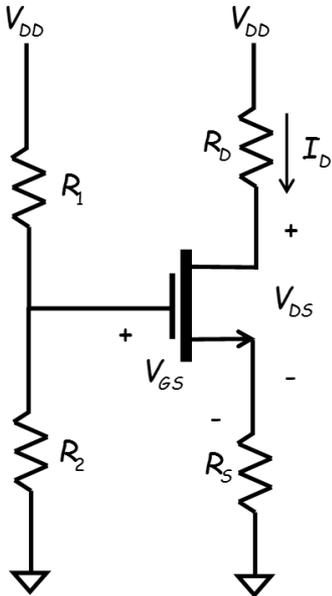
$$V_{DD} - I_D R_D - V_{DS} - I_D R_S = 0$$
