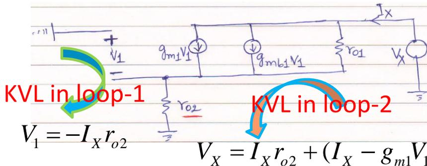
$$\Rightarrow \frac{V_X}{I_X} = r_{o2} + r_{o1} + r_{o1} (g_{m1} r_{o2} + g_{mb1} r_{o2}) = R_{out}$$
