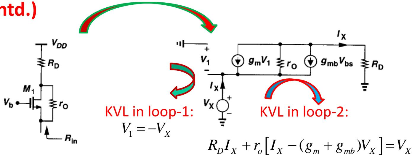
$$R_{in} = \frac{V_X}{I_X} = \frac{R_D + r_o}{1 + (g_m + g_{mb})r_o} \approx \frac{R_D}{(g_m + g_{mb})r_o} + \frac{1}{(g_m + g_{mb})}$$
