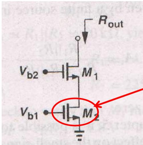
Gate and Source are fixed. Therefore this NFET works as a constant current source with an impedance  $r_{o2}$  across its drain and source
