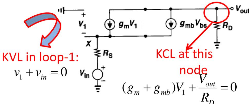
$$\Rightarrow A_v = \frac{V_{out}}{V_{in}} = (g_m + g_{mb})R_D = g_m(1 + \eta)R_D$$
