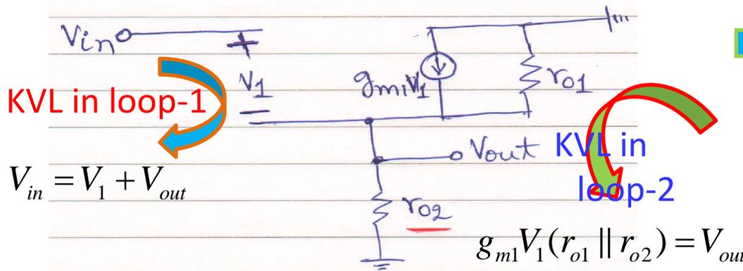
$$g_{m1} (V_{in} - V_{out}) (r_{o1} \parallel r_{o2}) = V_{out}$$
