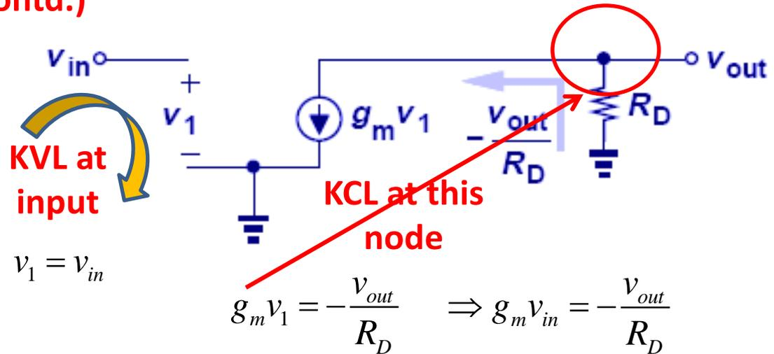
$$\therefore A_v = \frac{v_{out}}{v_{in}} = -g_m R_D$$
