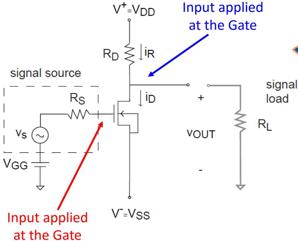
If the input is applied to the gate and the output is sensed at the drain, the circuit is called a "common-source" (CS) stage.
