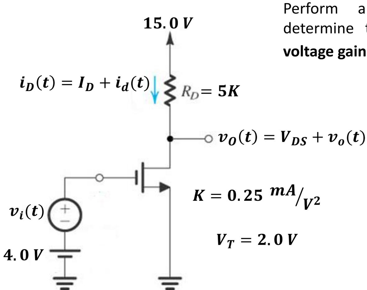
Perform a small-signal analysis to determine the small-signal open-circuit voltage gain  $A_v = v_o(t)/v_i(t)$
