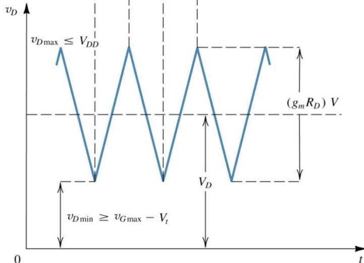
The input has been assumed very small as compared to overdrive voltage [ $v_{gs} \ll 2(V_{GS} - V_T)$ ]
