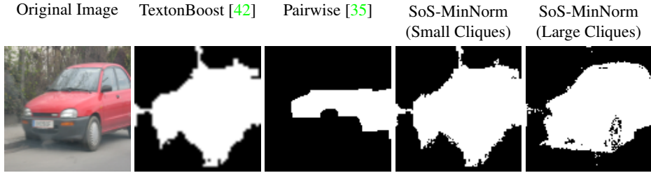
Figure 1: Pixel level object detection: We generate per pixel confidence using the probabilities generated by TextonBoost [42]. The second column titled TextonBoost has been generated based upon these confidence alone. The third column, shows the results using cliques of size of 2 only [35]. For generating higher order cliques to be used with our algorithm, we use region growing as suggested by Stobbe and Krause [44]. The fourth column shows the results using our algorithm with region growing restricted to 50 resulting in average clique size of 31. For testing with larger cliques, we allowed region growing until size 300 generating cliques with average size of 230. We used count based cost. The image size is 100 \times 100 and the time for small and large cliques is 0.6 and 53 seconds respectively. The quality of results seems to improve with increasing clique size.
