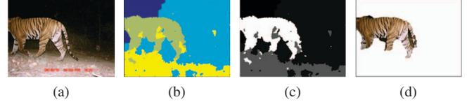
**Fig. 2:** Steps involved in Segmentation. (a) Test Image (b) Mean Shift Segmentation (different colors denote different clusters). (c) Distance Map (d) Segmentation Result after morphological operations on cluster with minimum distance
