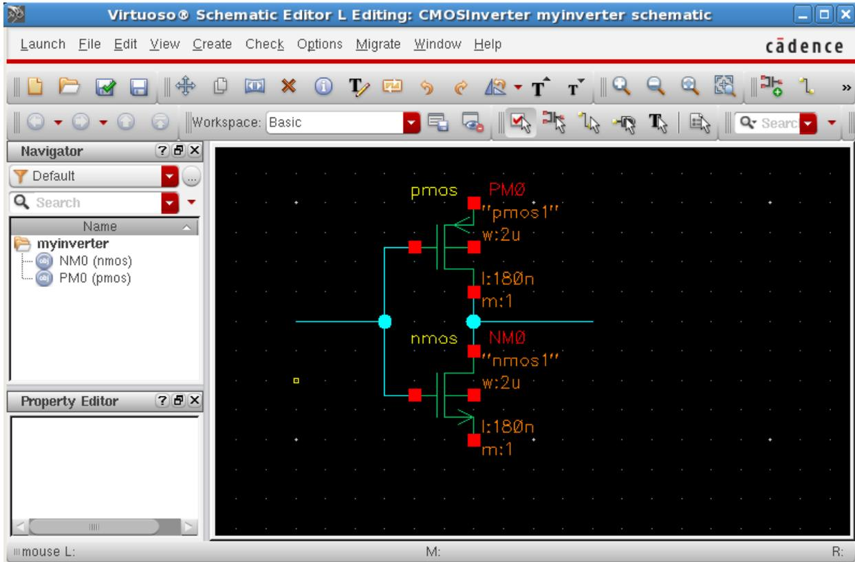
Fig 9 CMOS with no pins
