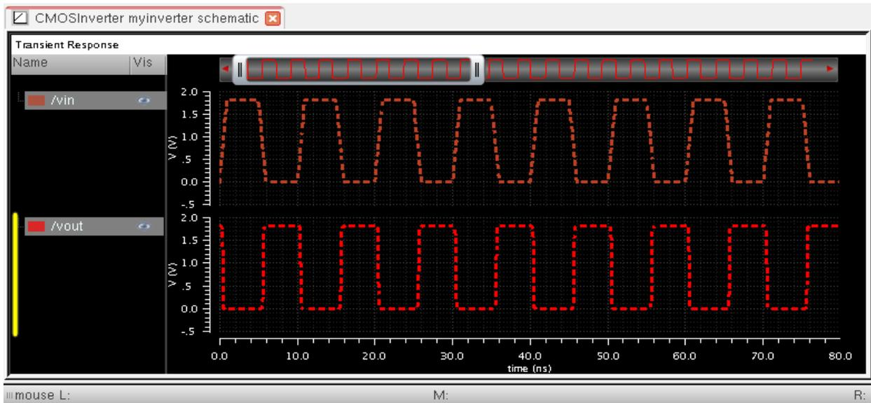
Fig. 18 Simulation Results (Transient Analysis)
