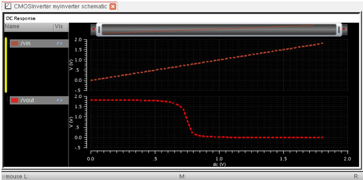
Fig. 17 Simulation Results (DC analysis)
