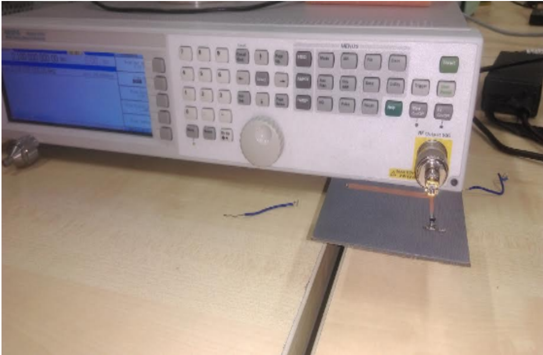
Figure 3.6: Prototype connected to Signal Generator
