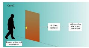
Figure 1. System response when presence detected near door
