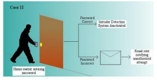
Figure 2. System response when password mechanism is used
