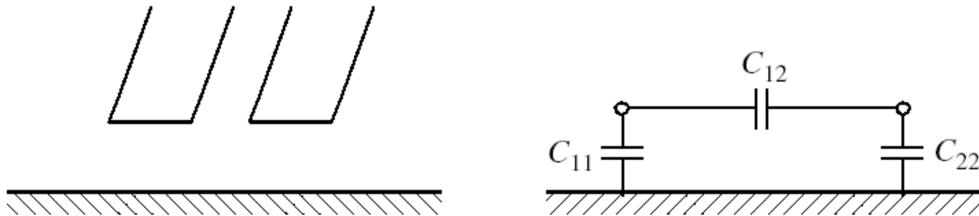
A three-wire coupled transmission line and its equivalent capacitance network
