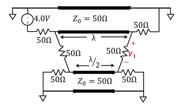
Use odd-even mode analysis to determine the value of voltage  $V_1$ .
