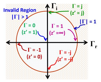
Apparently the normalized impedances can be mapped on complex  $\Gamma$ -plane and vice versa and gives us a clue that whole impedance contours (i.e, set of points) can be mapped to complex  $\Gamma$ -plane
