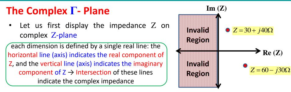
How do we plot an **open circuit** (i.e,  $Z = \infty$ ), **short circuit** (i.e, Z = 0), and **matching condition** (i.e,  $Z = Z_0 = 50\Omega$ ) on the complex Z-plane
