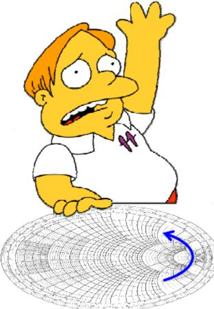
**Q:** Wait! I just used a Smith Chart to analyze a TL problem in the manner you have just explained. At one point on my transmission line the phase of the reflection coefficient is  $\theta_{\Gamma} = +170^{\circ}$ , which is denoted as 0.486 $\lambda$  on the "wavelengths toward load" scale.
