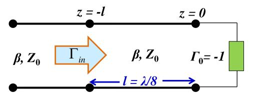
The reflection coefficient of a **short** circuit is  $\Gamma_0 = -1 = 1^* e(j\pi)$ , and therefore we **begin** at the leftmost point on the complex  $\Gamma$ -plane. We then move along a **circular arc**  $-2\beta l =$  $-2(\pi/4) = -\pi/2$  radians (i.e., rotate **clockwise** 90°).
