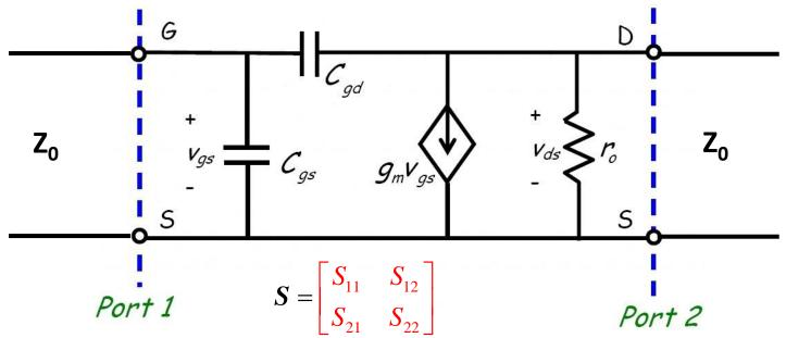
• We can determine this scattering matrix either by direct **measurement** (using a network analyzer) or by **analysis** of the small-signal circuit.
