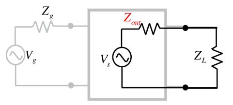
These four power quantities depend (at least in part) on the **source** parameters V<sub>g</sub> and Z<sub>g</sub>, **load** Z<sub>L</sub>, and the **scattering parameters** S<sub>11</sub>, S<sub>21</sub>, S<sub>22</sub>, S<sub>12</sub> of the gain element.
