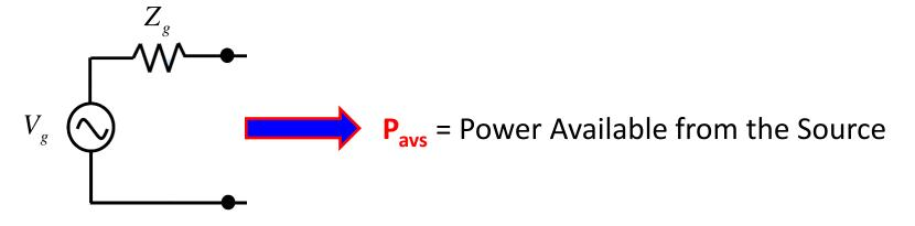
We likewise consider the power P<sub>in</sub> delivered by the source; in other words the power absorbed by the input impedance of the gain element with a load attached:
