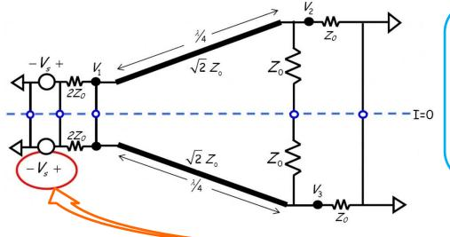
Note the **value** of the voltage sources. They have a value of  $V_s$  (as **opposed** to, say,  $2V_s$  or  $V_s/2$ ) because two equal voltage sources in **parallel** is equivalent to one voltage source of the **same value**.
