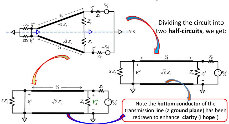
Analyzing the first half-circuit, we find that the transmission line is terminated in a short circuit in parallel with a resistor of value 2Z<sub>0</sub>. Thus, the transmission line is terminated in a short circuit!
