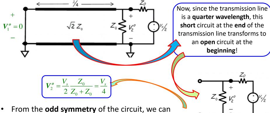
From the **odd symmetry** of the circuit, we can similarly determine:  $V_s^o = -\frac{V_s}{V_s^o}$
