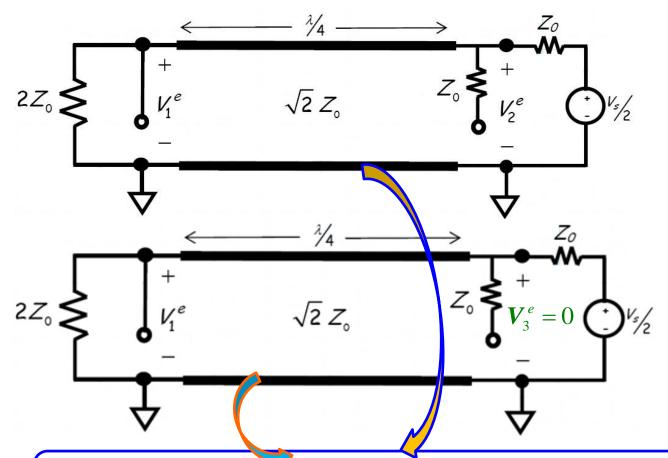
Note we have **again** drawn the **bottom conductor** of the transmission line (a **ground plane**).
