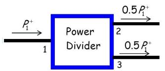
To efficiently divide the power incident Power 2 on the input port, the port (port 1)  $S_{11} = 0$  nust first be matched (i.e., all incident  $S_{11} = 0$ power should be delivered to port 1):
