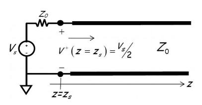
• Now, if the length of the transmission line connecting the source to a port (or load) is **electrically very small** (i.e.,  $\beta l << 1$ ), then the source is effectively **connected directly** to the source (i.e,  $\beta z_s = \beta z_p$ ):
