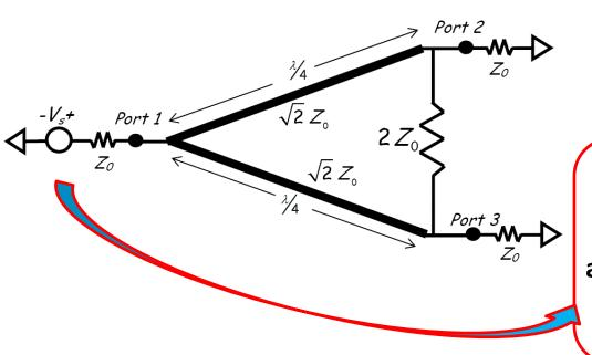
This source does **not** alter the bilateral symmetry of the circuit. We can thus use this symmetry to **help analyze** the circuit, **without** having to specifically define odd and even mode sources.
