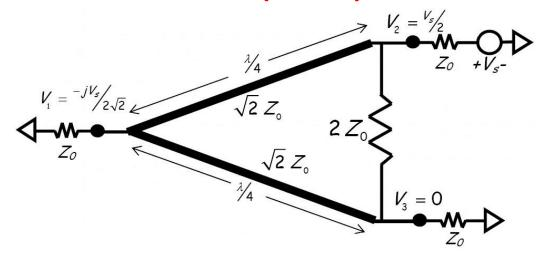
Note that the voltages we calculated are total voltages the sum of the incident and exiting waves at each port:
