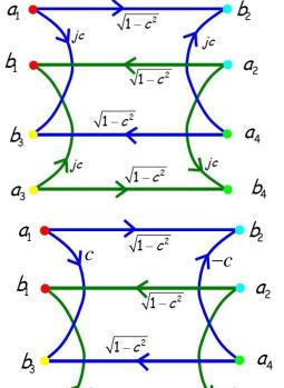
• Additionally, for a directional coupler, the coupling coefficient **c** will be **always** less than  $\frac{1}{\sqrt{2}}$ . Therefore, we can express:
