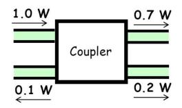
The **simplest** RF/microwave problem would seemingly be to **equally** divide signal power in two:
