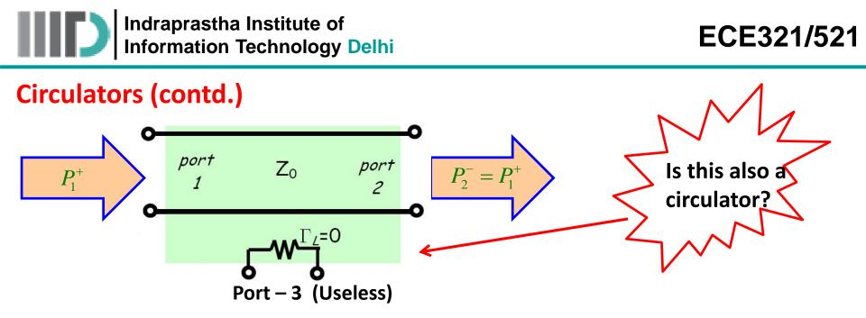
True! But a transmission line, being a reciprocal device, will likewise result in the power incident on port 2 of your simple circuit to exit completely from port 1 (P<sub>1</sub><sup>-</sup>=P<sub>2</sub><sup>+</sup>):
