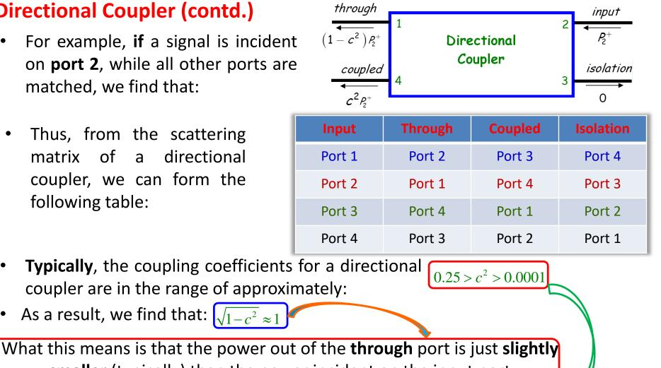
smaller (typically) than the power incident on the input port
