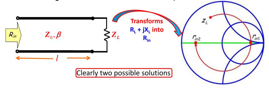
However, it should be understood that the input impedance will be purely real at only **one** frequency!
