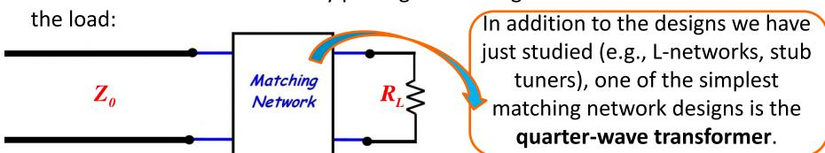
• The quarter-wave transformer is simply a transmission line with characteristic impedance  $Z_1$  and length  $l = \lambda/4$  (i.e., a quarter-wave line).
