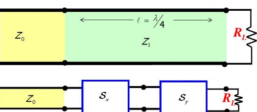
Q: Two two-port devices? It appears to me that a quarter-wave transformer is **not** that complex. What **are** the **two** two-port devices?
