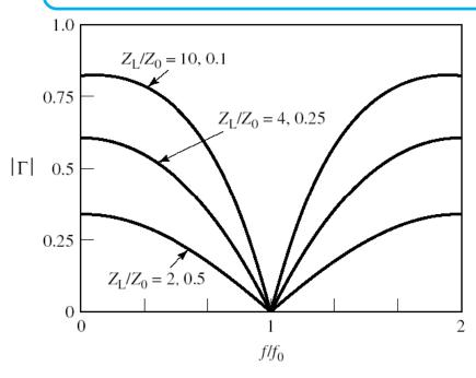
In principle, the bandwidth can be increased by adding multiple  $\lambda/4$  sections!
