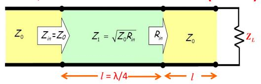
Again, since the transmission lines are lossless, **all** of the incident power is delivered to the **load**  $Z_L$ .
