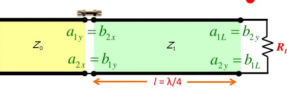
Therefore, we can put the signal-flow graph pieces together to form the signalflow graph of the quarter wave network:
