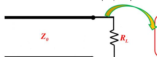
Unless  $R_L = Z_0$ , the resistor is **mismatched** to the line, and thus some of the incident power will be **reflected**.
