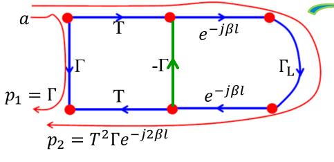
With respect to the theory of small reflections (where **only** direct paths are considered), this branch can be **removed** from the SFG **without affect**.
