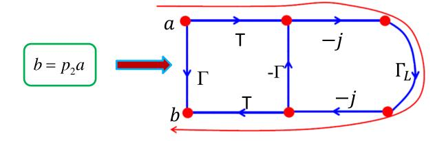
Path 3. However, a **portion** of this **second** wave is also **reflected** ( $\Gamma$ ) back into the Z<sub>1</sub> transmission line at z=-l, where it again travels by  $\beta l=90^{\circ}$  to the load, is partially reflected ( $\Gamma_L$ ), travels  $\beta l=90^{\circ}$  back to z=-l, and is partially transmitted into Z<sub>0</sub>(T)—our **third** reflected wave!
