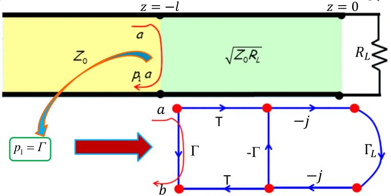
Path 2. However, a **portion** of the incident wave is transmitted (T) across the interface at z=-l, this wave travels a distance of  $\beta l=90^{\circ}$  to the load at z=0, where a portion of it is reflected ( $\Gamma_L$ ). This wave travels back  $\beta l=90^{\circ}$  to the interface at z=-l, where a portion is again transmitted (T) across into the  $Z_0$  transmission line—another reflected wave !
