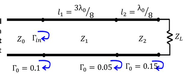
Note that the transmission line sections have **different lengths**!
