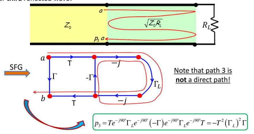
Path n. We can see that this "bouncing" back and forth can go on **forever**, with each trip launching a **new** reflected wave into the  $Z_0$  transmission line.
