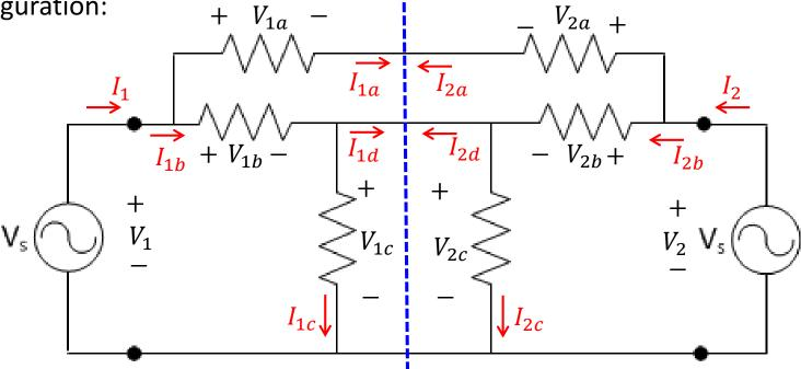
Since this circuit possesses bilateral (reflection) symmetry (1→2, 2→1), symmetric currents and voltages must be equal:
