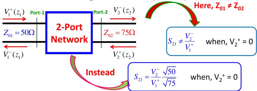
Note that the generalized scattering parameters can be more compactly written in terms of our new wave amplitude notation:
