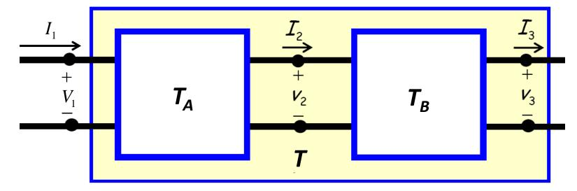
$$\left\{ \begin{matrix} V_1 \\ I_1 \end{matrix} \right\} = \boldsymbol{T}_{\boldsymbol{A}} \left\{ \begin{matrix} V_2 \\ I_2 \end{matrix} \right\}$$
