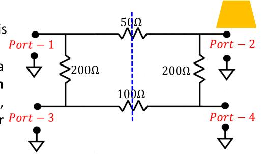
Continuing for all elements of the permutation, we find that for this symmetric circuit, the scattering matrix must have this form:
