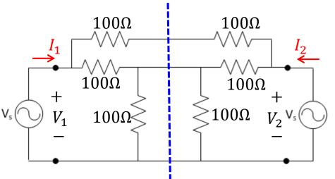
But remember! In order for **symmetry to be preserved**, the source values on both sides (i.e, V<sub>s</sub>) must be **identical**!
