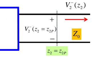
The complex ratio between  $V_1^+(z_1 = z_{1P})$  and  $V_2^-(z_2 = z_{2P})$  is known as the **scattering parameter**  $S_{21}$  Indraprastha Institute of Information Technology Delhi
