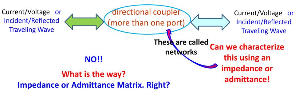
In principle, N by N impedance matrix completely characterizes a linear Nport device. Effectively, the impedance matrix defines a multi-port device the way a Z<sub>L</sub> describes a single port device (e.g., a load)
