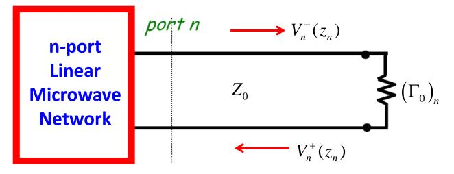
• For this current case, the situation is **reversed**. The wave incident on the load is **now** denoted as  $V_n^{-}(z_n)$  (coming **out** of port n), while the wave reflected off the load is **now** denoted as  $V_n^{+}(z_n)$  (going **into** port n).
