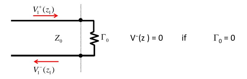
In this original case, the wave **incident** on the load is V<sup>+</sup>(z) (**plus** direction), while the **reflected** wave is V<sup>-</sup>(z) (**minus** direction).
