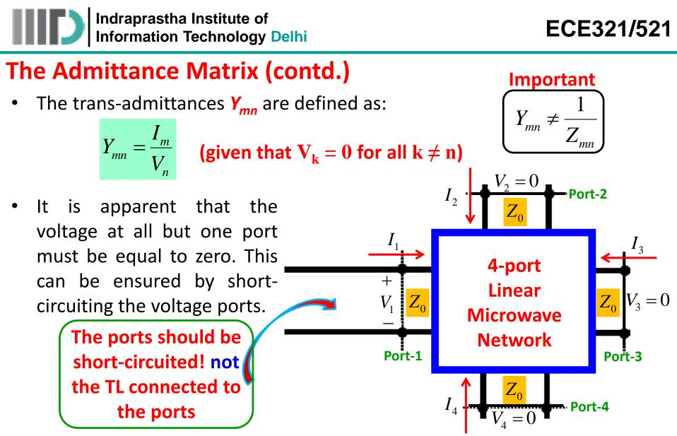
Now, since the network is linear, the current at any one port due to all the port voltages is simply the coherent sum of the currents at that port due to each of the port voltages.
