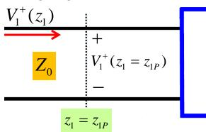
Say we measure/determine the voltage of the wave flowing **into port 1**, at the port 1 **plane** (i.e., determine  $V_1^+(z_1 = z_{1P})$ ).
