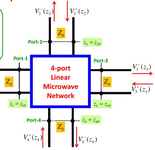
Viewing transmission line activity this way, we can fully characterize a multi-port device by its scattering parameters!
