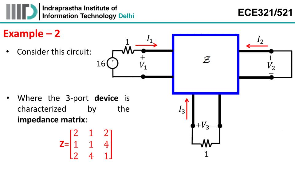
• determine all port **voltages** V<sub>1</sub>, V<sub>2</sub>, V<sub>3</sub> and all **currents** I<sub>1</sub>, I<sub>2</sub>, I<sub>3</sub>.
