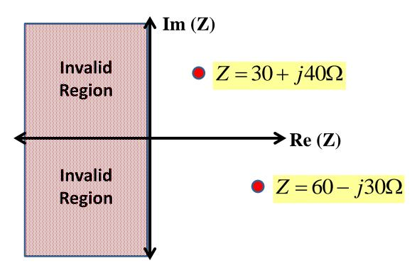
Note that each dimension is defined by a single real line: the horizontal line (axis) indicates the real component of Z, and the vertical line (axis) indicates the imaginary component of Z → Intersection of these lines indicate the complex impedance
