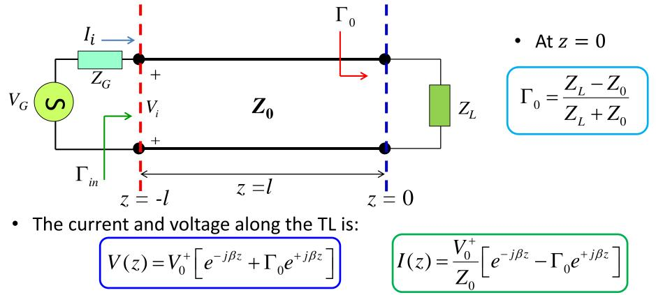
$V_0^+$  depends on the signal **source**! To determine its exact **value**, we must now apply **boundary conditions** at z = -l.
