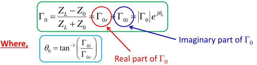
• In the special terminated conditions of pure short-circuit and pure opencircuit conditions the corresponding  $\Gamma_0$  are -1 and +1 located on the real axis in the complex  $\Gamma$ -plane.
