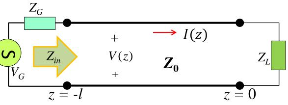
A: We of course **could** determine  $V_0^+$  and  $V_0^-$ , and then determine the power absorbed by the load (P<sub>abs</sub>) as:
