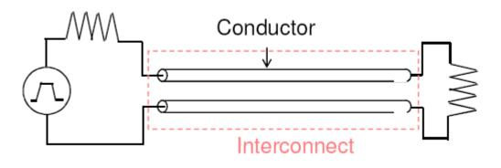
Therefore cables, wires, conductive tracks on printed circuit boards (PCBs), sockets, packaging, metallic tubes etc are all examples of interconnect.
