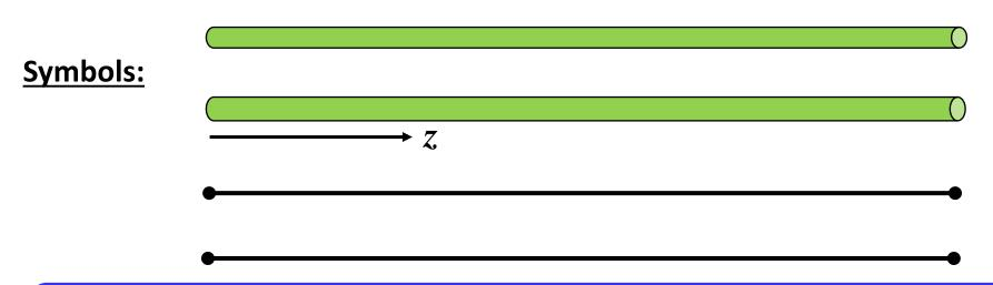
Note: We use this schematic to represent a general transmission line, no matter what the actual shape of the conductors.
