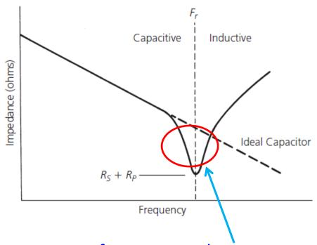
Presence of resonance due to dielectric loss and finite lead wires
