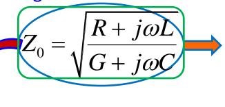
The incoming and outgoing voltage and current waves are position dependent → the ratio of voltage and current waves are independent of position → actually is a constant → an important characteristic of a transmission line → called as Characteristic Impedance
