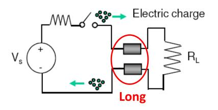
Electric charges move from  $V_s$  to the  $R_L$ . As the charge move, there is an associated EM field which travels along with the charges
