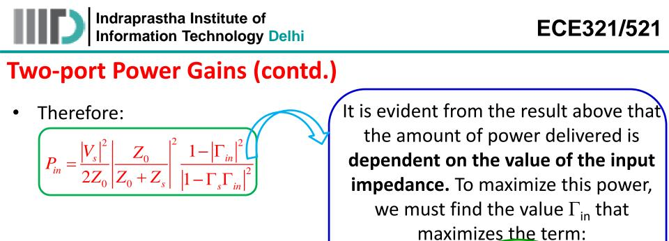
$P_{avs} = P_{in} |_{\Gamma_{in} = \Gamma_s^*} = \frac{|V_s|^2}{8Z_0} \frac{|1 - \Gamma_s|^2}{1 - |\Gamma|^2} = \frac{|V_s|^2}{2} \frac{1}{4 \operatorname{Re}\{Z_s^*\}}$
