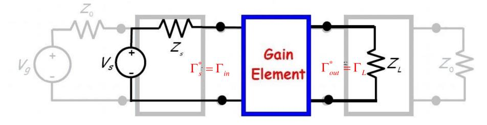
The values of  $\Gamma_s$  and  $\Gamma_l$  depend on the input and output matching networks
