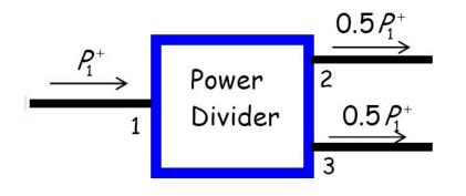
To efficiently divide the power incident on the input port, the port (port 1) must first be matched (i.e., **all incident power** should be delivered to port 1):  $S_{11} = 0$
