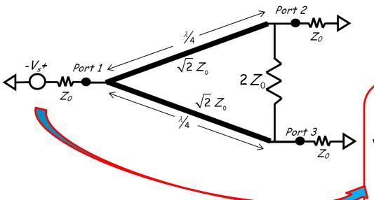
This source does **not** alter the bilateral symmetry of the circuit. We can thus use this symmetry to **help analyze** the circuit, **without** having to specifically define odd and even mode sources.
