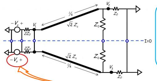
Note the **value** of the voltage sources. They have a value of V<sub>s</sub> (as **opposed** to, say, 2V<sub>s</sub> or V<sub>s</sub>/2) because two equal voltage sources in **parallel** is equivalent to one voltage source of the **same value**.
