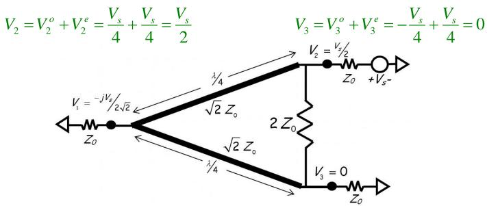
Note that the voltages we calculated are total voltages—the sum of the incident and exiting waves at each port:
