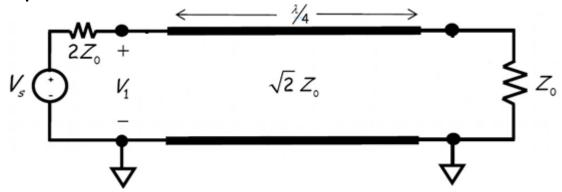
• Transforming the load resistor at the end of the  $\lambda/4$  line back to the start:
