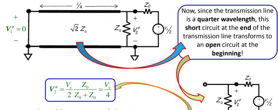
From the **odd symmetry** of the circuit, we can similarly determine:  $V^{o} - V_{s}$
