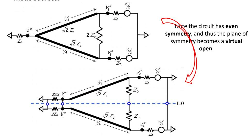
Dividing the circuit into two half-circuits, we get:
