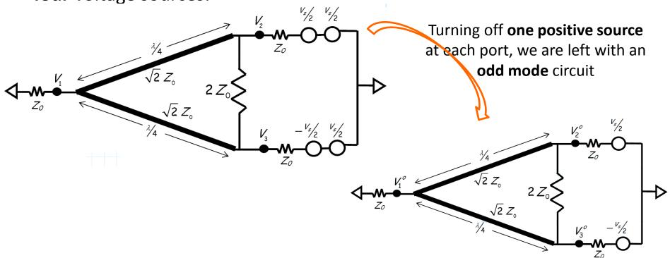
Note the circuit has odd symmetry, and thus the plane of symmetry becomes a virtual short, and in this case, a virtual ground!
