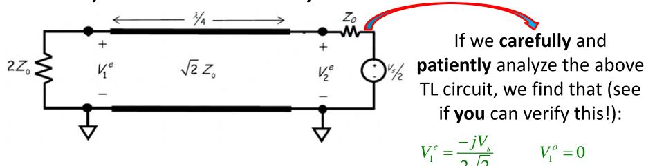
This completes our symmetry analysis and then from superposition, the voltages within the circuit is simply found from the sum of the solutions of each mode:
