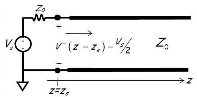
• Now, if the length of the transmission line connecting the source to a port (or load) is **electrically very small** (i.e.,  $\beta l << 1$ ), then the source is effectively **connected directly** to the source (i.e,  $\beta z_s = \beta z_p$ ):
