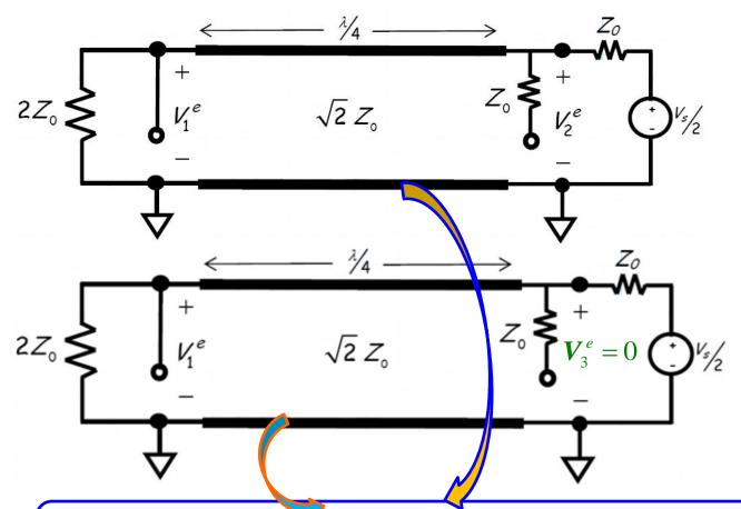
Note we have **again** drawn the **bottom conductor** of the transmission line (a **ground plane**).
