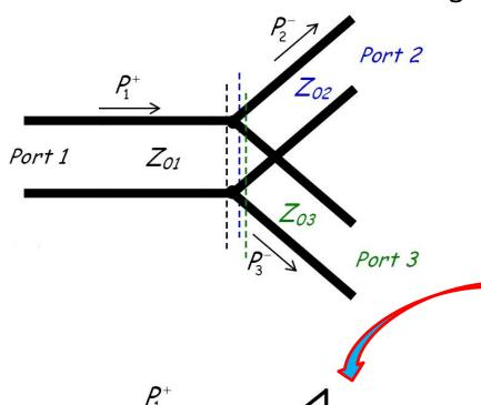
To be ideal, we want  $S_{11} = 0$ . Thus, when **ports 2** and **port 3** are **terminated** in matched loads, the input impedance at **port 1** ( $Z_{01}$ ) must be related to impedances  $Z_{02}$  and  $Z_{03}$  as:
