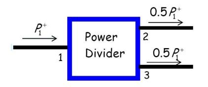
To efficiently divide the power incident on the input port, the port (port 1) must first be matched (i.e., **all incident power** should be delivered to port 1):
