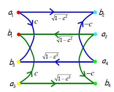
• Additionally, for a directional coupler, the coupling coefficient c will be **always** less than  $\frac{1}{\sqrt{2}}$ . Therefore, we can express:
