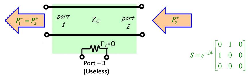
But, this is **not true for a circulator! If power is incident on** port 2, then **no power will exit port 1!**
