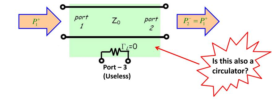
• True! But a transmission line, being a **reciprocal device**, will likewise result in the power **incident on port 2 of your simple** circuit to **exit completely from port 1** ( $P_1^-=P_2^+$ ):
