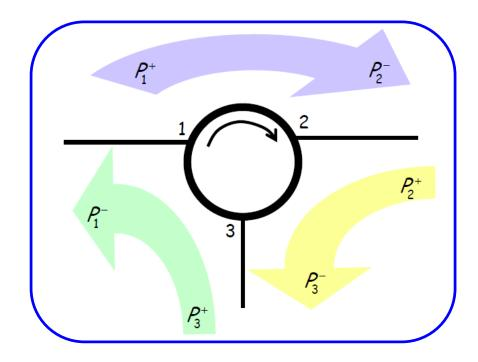
We can see that, for example, a source at port 2 "thinks" it is attached to a load at port 3, while a load at port 2 "thinks" it is attached to a source at port 1!
