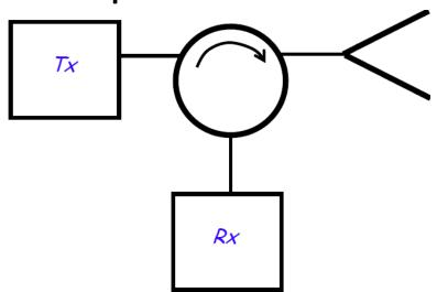
It is particularly important to keep the transmitter power from getting to the receiver. To accomplish this, the antenna must be matched to the transmission line. Do you see why?
