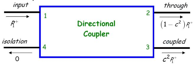
Note however, that **any** of the coupler ports can be an input, with a **different** through, coupled and isolation port for each case
