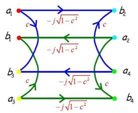
**5)** Reduce this signal flow graph for the case where ports 2, 3, and 4 are terminated in **matched loads** ( $\Gamma_{L2} = \Gamma_{L3} = \Gamma_{L4} = 0$ ), and determine **in decibels** the numeric value of  $|S_{11}|^2$ ,  $|S_{21}|^2$ ,  $|S_{31}|^2$ , and  $|S_{41}|^2$ , at the **design frequency**. Q2: Do these values precisely match those provided by the ADS analysis? Why or why not?
