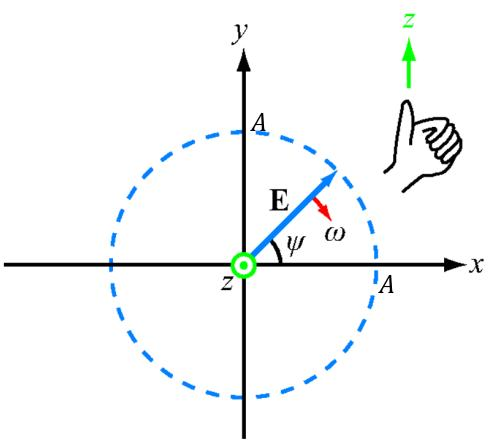
When the thumb of the left hand points along the direction of propagation (the z - direction in this case), the other four fingers point in the direction of rotation of  $\vec{E}$ .
