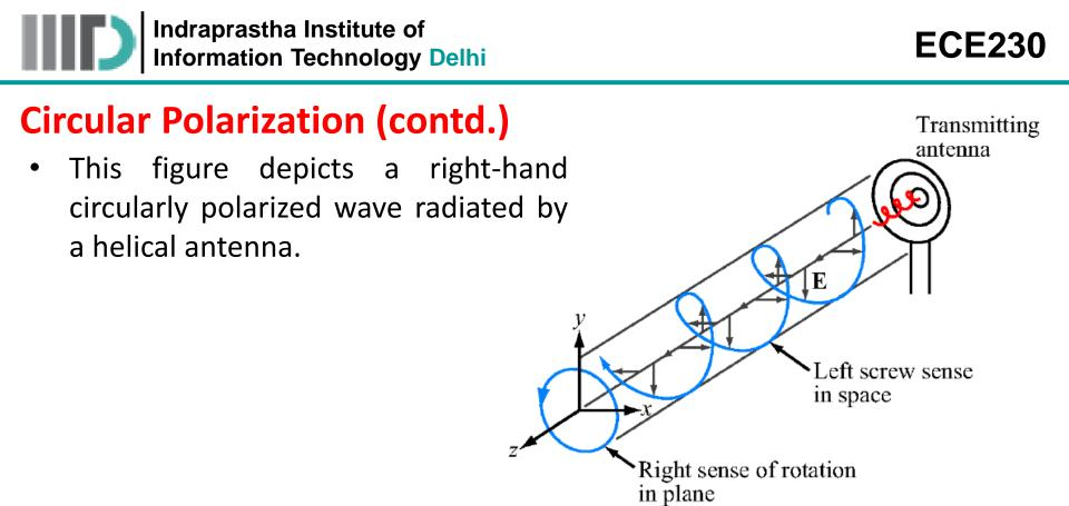
Polarization handedness is defined in terms of the rotation of  $\vec{E}$  as a function of time in a fixed plane orthogonal to the direction of propagation, which is opposite to the direction of rotation of  $\vec{E}$  as a function of distance at a fixed point in time.
