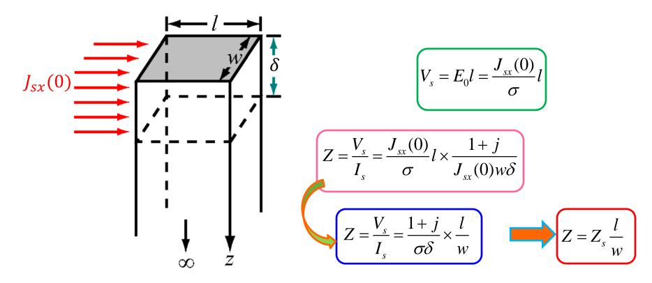
$Z_s$  is surface impedance and the real part of this is called ac resistance.
