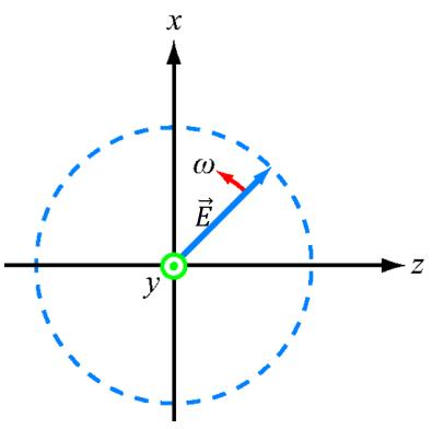
• Let us assign the z-component of  $\vec{E}_s(y)$ a phase angle of zero and the xcomponent a phase shift of  $\delta_p = -\frac{\pi}{2}$ .
