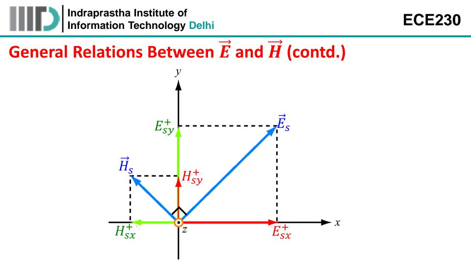
In general, a TEM wave may have an electric field in any direction in the plane orthogonal to the direction of wave travel, and the associated magnetic field is also in the same plane with appropriate magnitude and direction.
