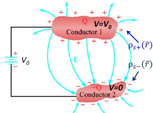
• Likewise, if there is an electric field, then we can specify an **electric flux density**  $\vec{D}(\vec{r})$ , which we can use to determine the **surface charge density**  $\rho_s(\vec{r})$  on each of the conductors.
