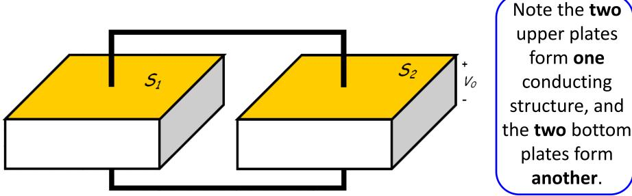
Q: What is the **capacitance** between these two conducting structures? A: The potential difference between them is V<sub>0</sub>. The **total charge** on one
