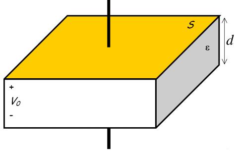
Recall that we determined the fields and surface charge density of an **infinite** pair of parallel plates. We can use those results to approximate the fields and charge densities of this **finite** structure, where the **area** of each plate is *S*.
