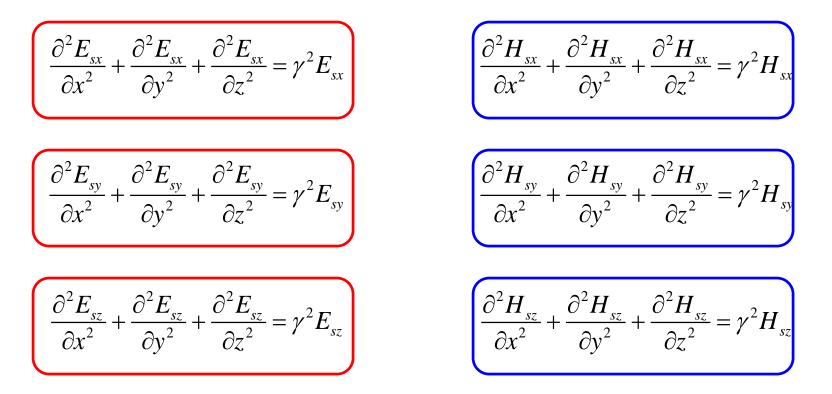
The component fields of any time-harmonic EM wave must individually satisfy these six partial differential equations. In many cases, the EM wave will not contain all six components. An example of this is the *plane wave*.
