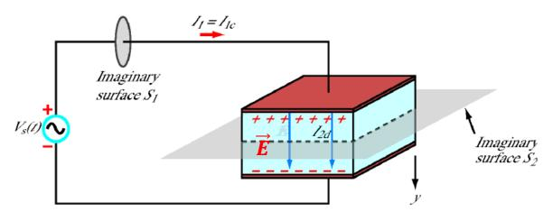
Let us find  $I_c$  and  $I_d$ through each of the two imaginary surfaces: (1) cross section of the conducting wire,  $S_1$ ; (2) cross section of the capacitor,  $S_2$ .
