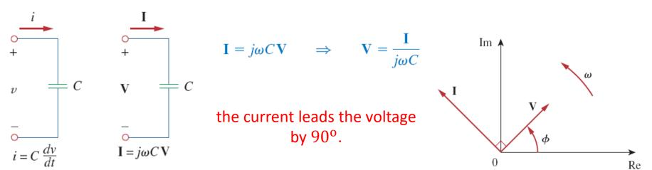
What is the instantaneous voltage across a  $2\mu$ F capacitor when the current through it is  $i = 4 \sin(10^6 t + 25^\circ) A$ ?
