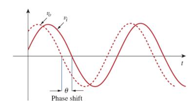
the circuit current I leads the applied voltage by some phase angle  $\theta$ , where  $0 < \theta < 90^{\circ}$ depending on the values of *R* and *C*.
