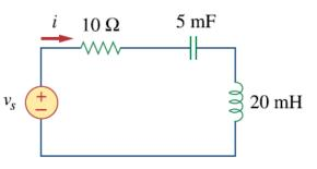
Find current *i* in this circuit, when  $v_s(t) = 60\cos(200t - 10^\circ)$  V.
