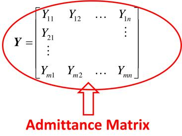
$$\begin{bmatrix} I_{3} = Y_{34}V_{4} + Y_{33}V_{3} + Y_{32}V_{2} + Y_{31}V_{1} \\ I_{m} = \sum_{n=1}^{N} Y_{mn}V_{n} \implies \implies \mathbf{I} = \mathbf{Y}\mathbf{V} \\ \Rightarrow \mathbf{I} = \begin{bmatrix} \mathbf{I}_{1}, \mathbf{I}_{2}, \mathbf{I}_{3}, \dots, \mathbf{I}_{N} \end{bmatrix}^{T}$$
