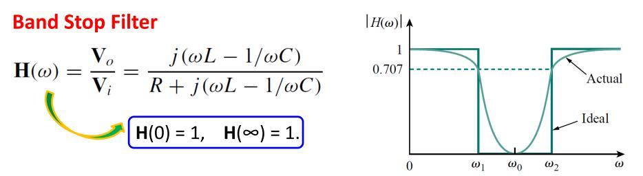
• But at resonance frequency:  $v_0 = 0 \Rightarrow$  Filters blocks  $\omega_0$
