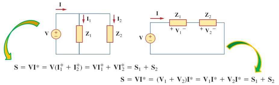
whether the loads are connected in series or in parallel (or in general), the total power *supplied* by the source equals the total power *delivered* to the load
