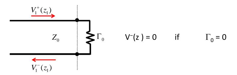
In this original case, the wave **incident** on the load is  $V^+(z)$  (**plus** direction), while the **reflected** wave is  $V^-(z)$  (**minus** direction).
