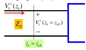
Say we measure/determine the voltage of the wave flowing **into port 1**, at the port 1 **plane** (i.e., determine  $V_1^+(z_1 = z_{1P})$ ).
