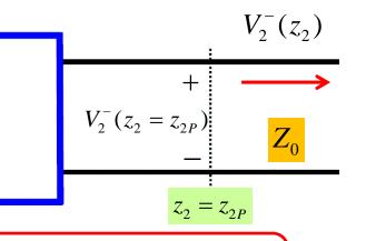
The complex ratio between  $V_1^+(z_1 = z_{1P})$  and  $V_2^-(z_2 = z_{2P})$  is known as the **scattering parameter**  $S_{21}$
