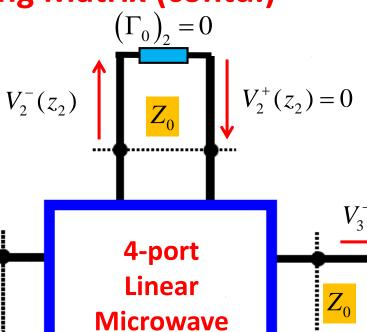
Note that **if** the ports are terminated in a **matched load** (i.e.,  $Z_L = Z_0$ ), then  $(\Gamma_0)_n = 0$  and therefore:
