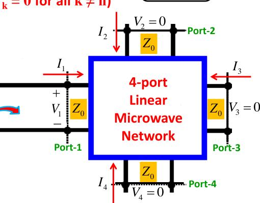
Now, since the network is linear, the current at any one port due to all the port voltages is simply the coherent sum of the currents at that port due to each of the port voltages.
