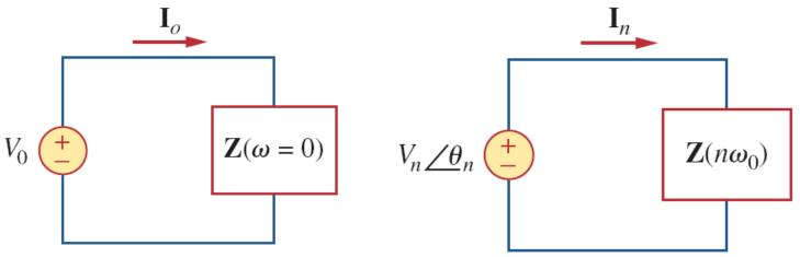
The network is represented by its impedance  $\mathbf{Z}(n\omega_0)$  and it's the value when  $\omega$  is everywhere replaced by  $n\omega_0$
