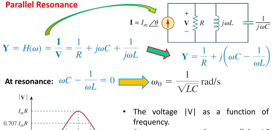
At resonance, the parallel *LC* combination acts like an open circuit, so that the entire current flows through *R*.
