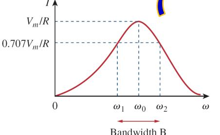
A metric known as *quality factor Q* relates the maximum or peak energy stored to the energy dissipated in the circuit per cycle of oscillation. The height of the curve is determined by *R*, the width of the curve depends on the *bandwidth B* defined as:
