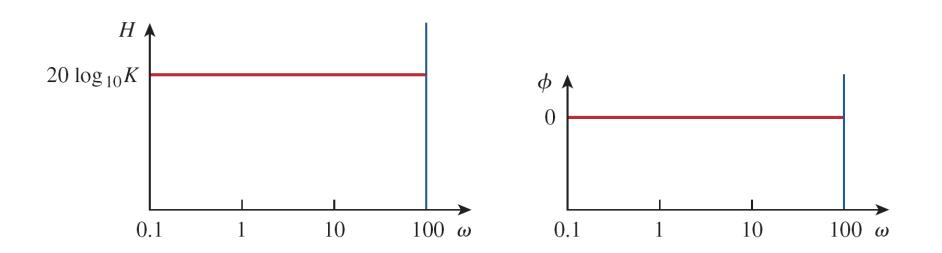
For negative K, the magnitude remains  $20log_{10}|K|$  but the phase angle is  $\pm 180^{\circ}$
