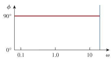
The Bode plots for the pole  $(j\omega)^{-1}$  are similar except that the slope of the magnitude plot is -20dB/decade while the phase is  $-90^{\circ}$ . In general, for  $(j\omega)^{N}$  where N is an integer, the magnitude plot will have a slope of 20N dB/decade, while the phase is 90N degrees.
