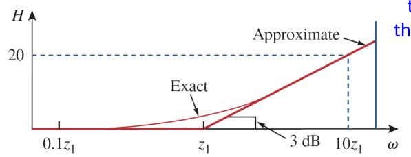
the approximate plot is close to the actual plot except at the break frequency ( $\omega=z_1$ ), where the deviation is  $20log_{10}|1+j1|=20log_{10}|\sqrt{2}|\approx 3dB.$
