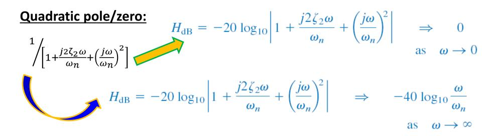
Clearly, the amplitude plot consists of two straight asymptotic lines: one with zero slope for  $\omega < \omega_n$  and the other with slope  $-40~dB/{\rm decade}$  for  $\omega > \omega_n$  with  $\omega_n$  as the corner frequency.
