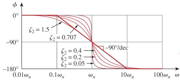
The phase plot is a straight line with a slope of  $-90^{\circ}$  per decade starting at  $\frac{\omega_n}{10}$  and ending at  $10\omega_n$
