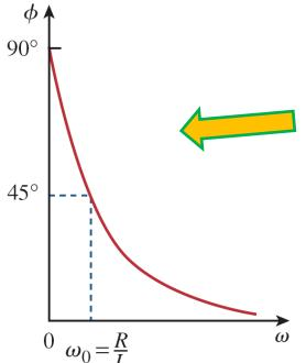
$$H(\omega) = \frac{V_0}{V_S} = \frac{j\omega L}{R + j\omega L}$$
