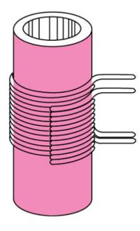
The air-core transformers used in radio frequency circuits are loosely coupled, whereas ironcore transformers used in power systems are tightly coupled.
