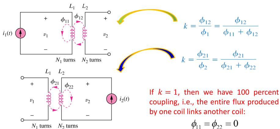
The coupling coefficient k is a measure of the magnetic coupling between two coils:  $0 \le k \le 1$
