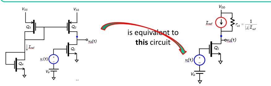
• The resulting small-signal circuit of this amp is:
