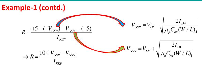
The resistor R can be replaced by an active load such as the PFET shown here → what will be its W/L?
