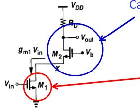
Cascode device (in CG)  $\rightarrow$  in saturation  $\rightarrow$  routes the current generated by main device to R<sub>D</sub>
