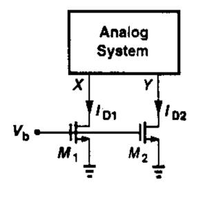
Q: determine the resulting difference between  $I_{D1}$  and  $I_{D2}$  if  $\lambda \neq 0$
