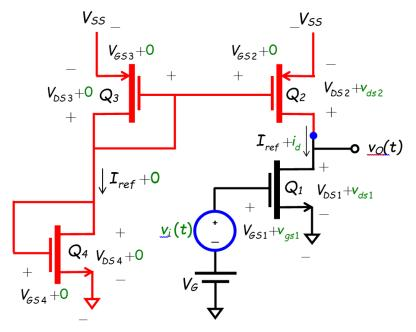
**Q:** But wait! **How** can there be a smallsignal **drain current**  $i_{d2}(t)$  through transistor Q<sub>2</sub>, without a corresponding small-signal  $v_{gs2}(t)$  gate-to-source voltage?
