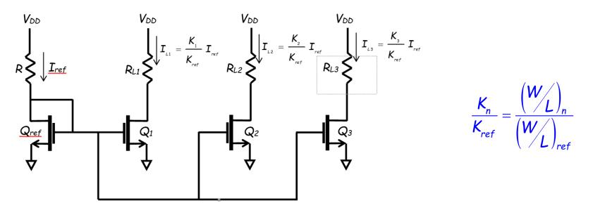
From the standpoint of integrated circuit design, we can change the value of K by modifying the MOSFET channel **width-tolength ratio** (W/L) for each transistor.
