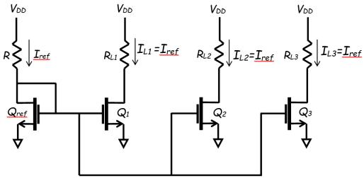
This circuit is particularly useful in integrated circuit design, where **one** resistor *R* is used to make **multiple** current sources.
