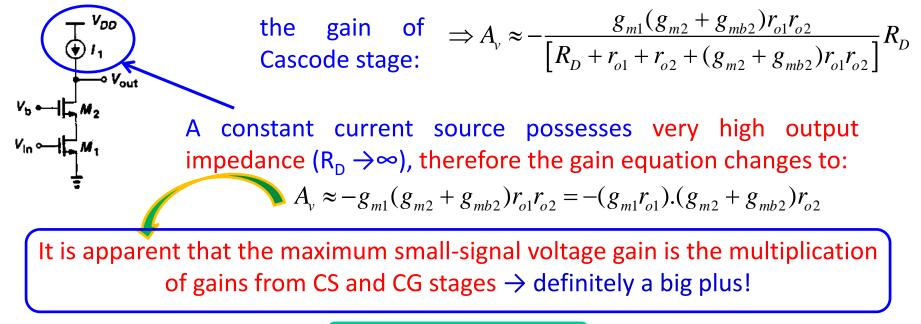
$$R_{out} \approx \left(g_{m2} + g_{mb2}\right) r_{o2} r_{o1}$$
