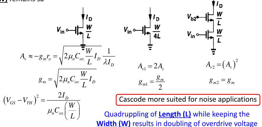
For identical devices, cascode also exhibits doubling of overdrive voltage
