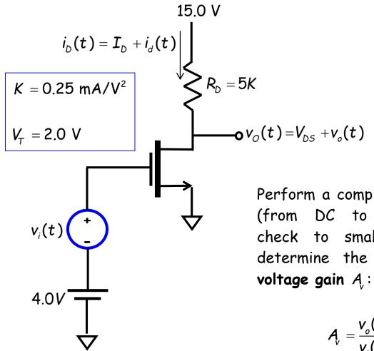
Perform a complete analysis (from DC to assumption check to small-signal) to determine the small-signal
