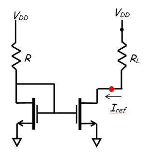
• Remember, the second MOSFET **must** be in saturation for the current through  $R_L$  to be a constant value  $I_{ref}$ . As a result, we find that:
