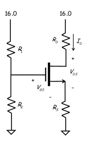
• If the MOSFET has device values  $K=1.0\ ^{mA}/_{V^2}$  and  $V_T=1.0V$ , determine the resistor values to bias this MOSFET with a DC drain current of  $I_D=4.0mA$ .
