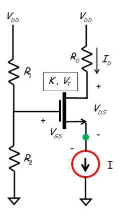
It is evident that the DC drain current  $I_D$ , is equal to the current source I, regardless of the MOSFET values K or  $V_T$ !
