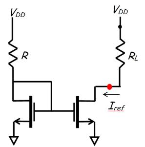
$$R_L < rac{V_{DD} - V_{G1} + V_{T1}}{I_{ref}}$$
